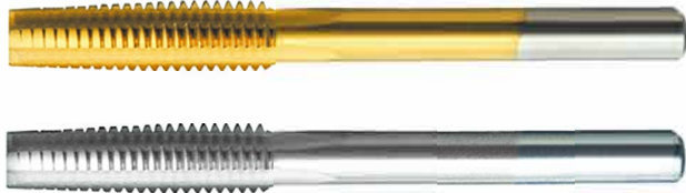
DIN357 机用螺母丝锥 DIN357 Machine Nut Taps DIN357,with metric-ISO thread DIN13,tolerance 6H=IS02 M2 HSS M35 HSS-E,Coating,available for specified requirements
